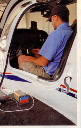
After removing the mechanical standby gauges, avionics technician lan Terry prepares to mount the Trilogy in their place. The Trilogy contains an internal AHRS and air data computer, and plugs into the same electrical, pitot, and static lines as the instruments it replaces. There's no need for new wires or probes.
