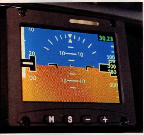
A Trilogy standby instrument makes the Let's Go Flying SR22 panel all glass. The airplane's mechanical back-up gauges (below) are gone for good.
